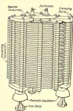
Fig. 249.—A current-limiting reactor.
